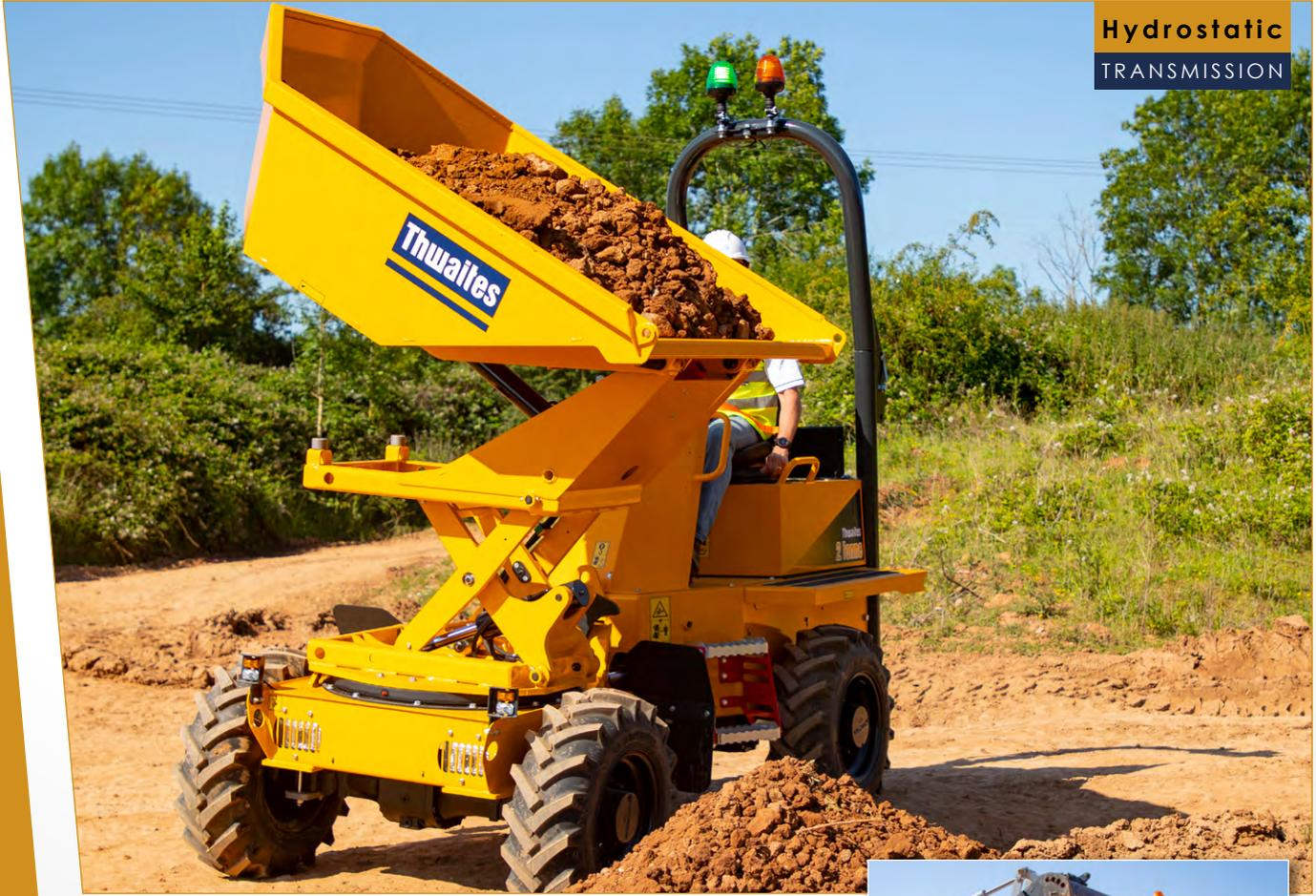
The Thwaites 2 Tonne Hi Swivel, Stage V dumper is manufactured with contractors and hirers in mind – ensuring operator safety, reducing risk on site and improving performance. Powered by an 18.1 kW 3-cylinder Yanmar engine, delivering 107 Nm max torque for optimum traction and control, this machine is driven by a Hydrostatic transmission, making it simple and straightforward to operate.
