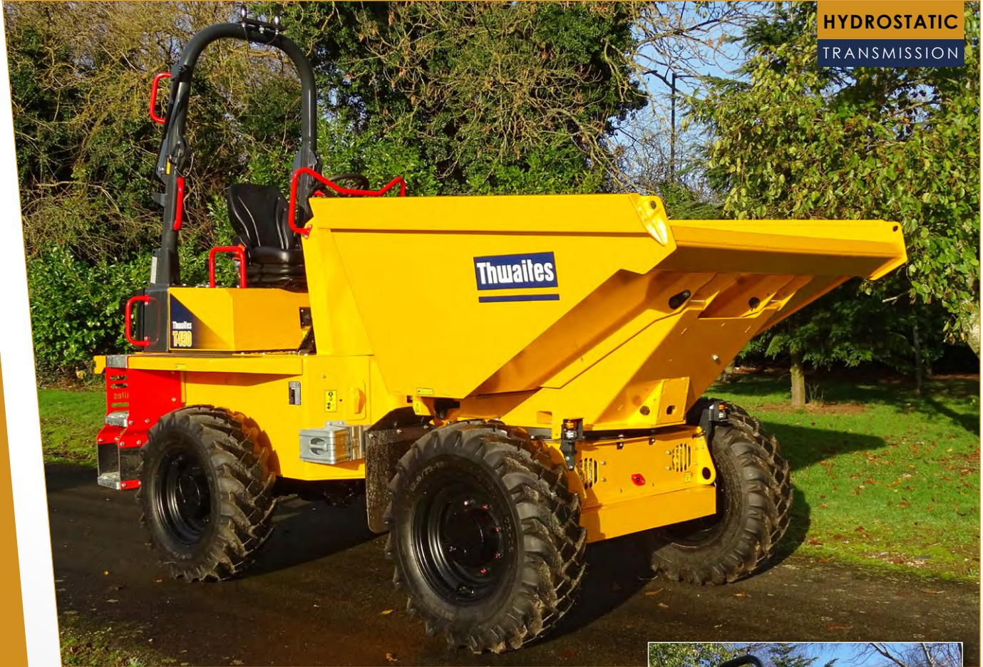
The Thwaites T450 Power Swivel, Stage V dumper is manufactured with contractors and hirers in mind – ensuring operator safety, reducing risk on site and improving performance. Powered by a 33.3 kW Yanmar engine, delivering 142 Nm max torque for optimum traction and control, this machine is driven by a Hydrostatic transmission, making it simple and straightforward to operate.
