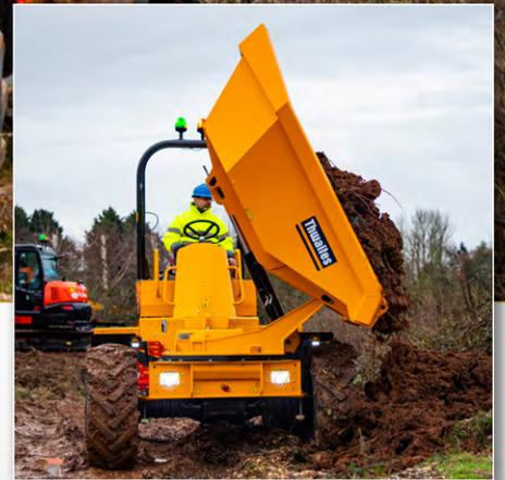
The Thwaites 6 Tonne Power Swivel, Stage V dumper is manufactured with contractors and hirers in mind – ensuring operator safety, reducing risk on site and improving performance. The Power Swivel skip enables a 90° rotation left and right, allowing the machine easier access to tip loads in restricted areas, giving the operator greater control and reducing risk on site.
